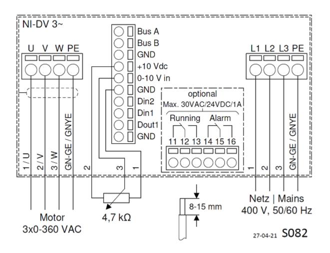
Wiring diagram for connection to: mains - VSD - motor Rotation: RD
